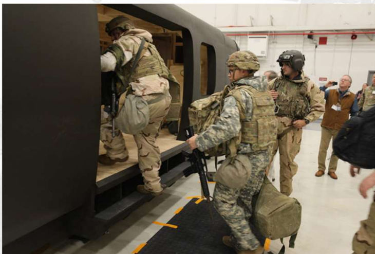
Soldiers entering the cabin mockup during Solder Engagement #1. An objective was to evaluate the step design for ingress & egress.
